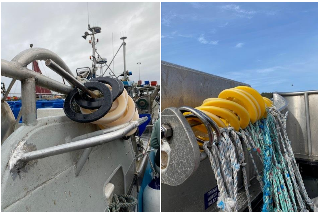
Figure 2. Dyneema (UHMWPE) purse rings by gannet nets ( https://www.gannetnets.com/ ) on two UoA vessels and by comparison a more traditional stainless steel purse ring (right image). Credit: CU UK
